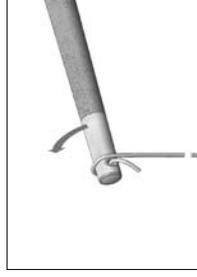
**Winding metal strings on the tapered tuning pin**
